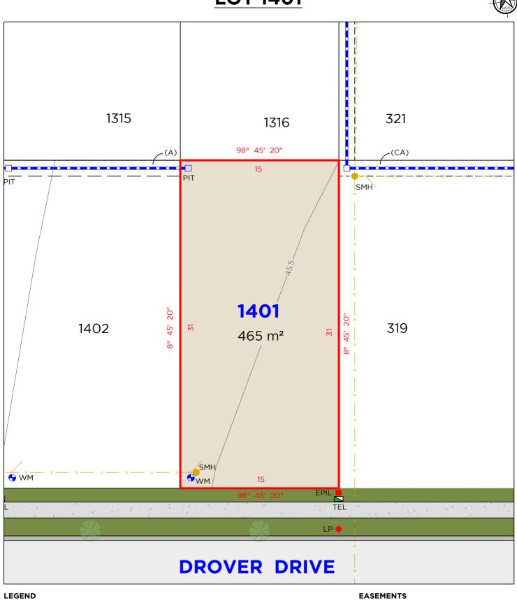
BOUNDARY LINE ADJACENT BOUNDARY EASEMENT SEWER STORMWATER
