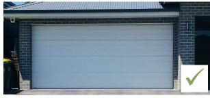
**GARAGING** - the garage door is not to be a dominant feature of the façade. The garage is to be a maximum of 50% of the width of the façade and is to be set-back a minimum of 1 meter from the main wall of the facade.
