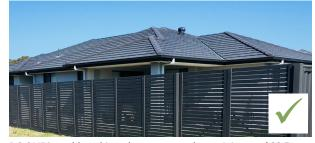
**ROOVES** – gable or hipped rooves are to be a minimum of 22.5 degrees pitch and skillion rooves a minimum of 10 degrees pitch. Roof materials are to be concrete tiles (flat profile preferred) or metal Colorbond Custom Orb. Roof colour is to be of a natural earth tone with a preference for dark 'grey' tones.
